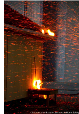
The broom on this test deck was ignited by wind-blown embers. Note that the embers also ignited pine needle debris in the gutter.
