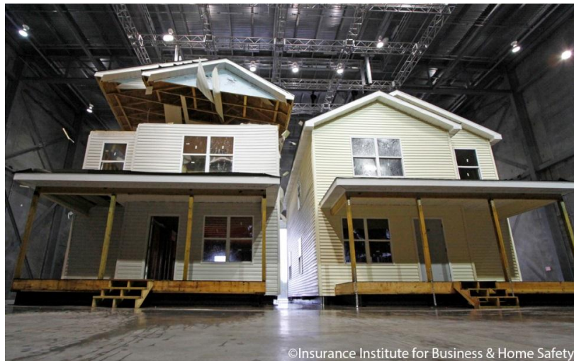
Figure 2: High wind test in the IBHS large test chamber. The home on the left was built to withstand gust wind speeds of 90 mph while the home on the right was built to the IBHS Fortified level and withstood more extreme wind conditions.
